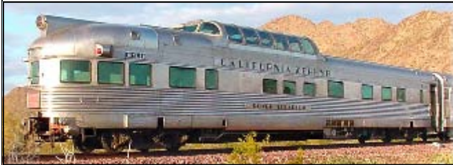
The 'Silver Solarium', Vista Dome observation sleeping car built by Budd in 1948 for the famous "California Zephyr."
